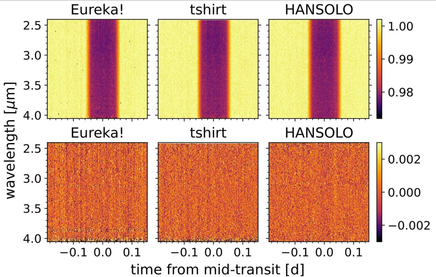
**Extended Data Fig. 6 | JWST's NIRCам data of WASP-39 as a function of time and wavelength for each independent reduction (top) and their residuals (bottom).** Top: time-series NIRCам data for the WASP-39b system, from three
