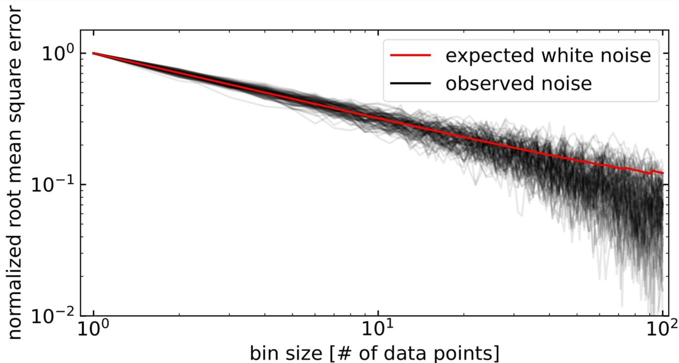
**Extended Data Fig. 4 | Normalized root-mean-square error as a function of bin size for all spectroscopic channels.** The red line shows the expected relationship for perfect Gaussian white noise. The black lines show the observed noise from each spectroscopic channel for the Eureka! long-wavelength reduction. Values for all channels are normalized by dividing by the value for a
