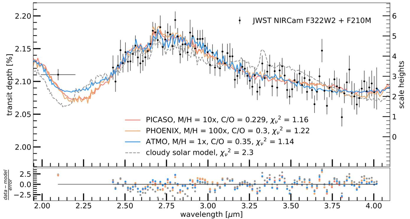
**Extended Data Fig. 7 | Measured transmission spectrum compared to atmospheric forward model grids.** Top: the single best fit for each model grid (shown as solid coloured lines; PICASO 3.0, ATMO, PHOENIX), fits the planet spectrum (Eureka! reduction) with  $\chi_\nu^2 \leq 1.22$ . All single best fits prefer at least solar metallicity and substantial cloud cover. Also shown as a grey dashed line is a solar metallicity, stellar C/O ratio atmospheric model, demonstrating the lack
