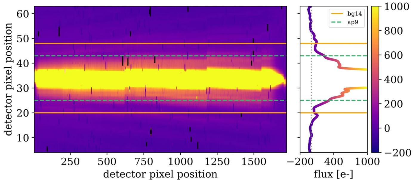
**Extended Data Fig. 3 | Median NIRCcam frame, after curvature correction and background subtraction, shown as the full 2D frame (left) and a vertical slice (right).** Left: curvature-corrected, background-subtracted, median frame. We perform optimal spectral extraction on the pixels in between the green dashed lines. We use the pixels outside of the two orange
