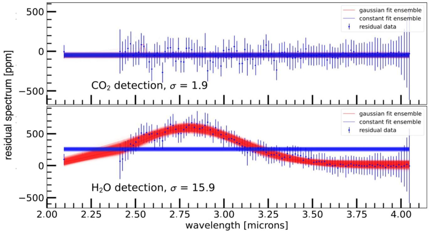
**Extended Data Fig. 9 | Gaussian residual fitting of H<sub>2</sub>O and CO<sub>2</sub>.** The blue points show the residual features left after subtracting out the gas in question (CO<sub>2</sub>, top, and H<sub>2</sub>O, bottom) from the single best-fit model. The Gaussian model
