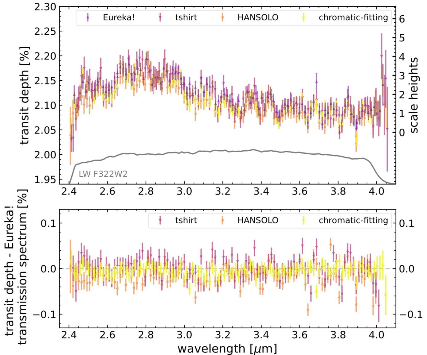
**Extended Data Fig. 5 | The transit spectrum of WSP-39b as determined by our independent analysis using JWST's NIRCam instrument (top) and the respective differences between our results (bottom).** Top: transmission spectra from our reductions when including additional data on the blue and red edges (now spanning 2.405–4.055  $\mu\text{m}$ ). This demonstrates the large error bars and diverging data points near the edges of the NIRCam bandpass in the
