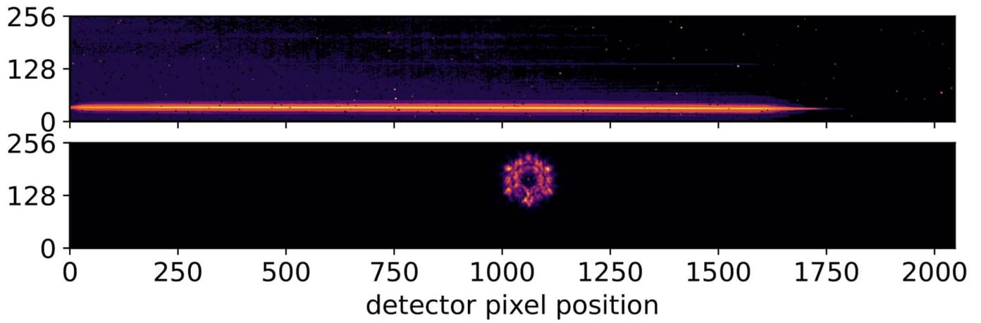
**Extended Data Fig. 2 | Raw NIRCams image of the LW (top) and SW (bottom) channels.** The faint horizontal stripes seen in the LW channel originate from neighbouring objects. The SW channel is able to track changes in alignment for individual mirror segments. No impactful tilt events were noted in this observation.
